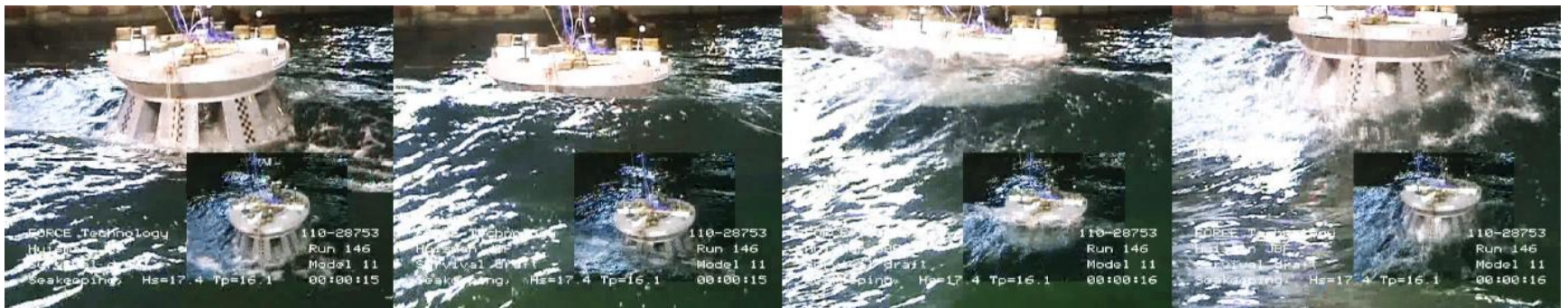
Model tests of JBF Arctic in irregular waves in survival condition meeting the wave H_{sig}=17.4\text{m}
