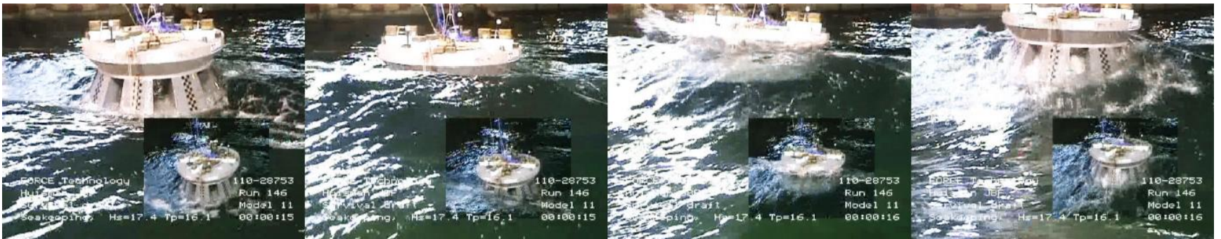
Model tests of JBF Arctic in irregular waves in survival condition meeting the wave H_{sig}=17.4m
