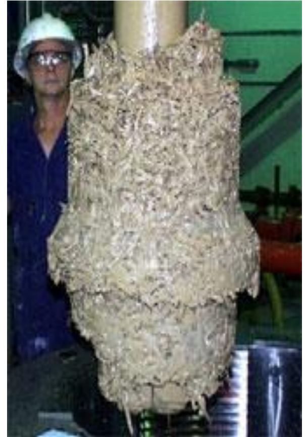
Adverse mud-shale reaction: bit-balling
