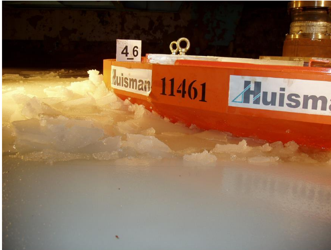
Model tests of JBF Arctic in ice (ice draft and transit draft)
