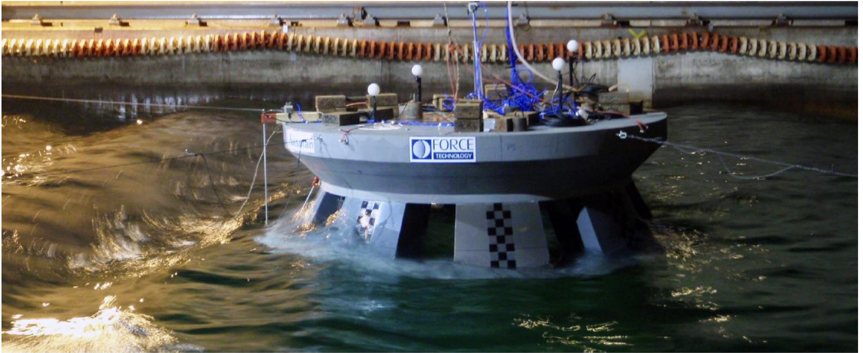
Model tests of JBF Arctic in irregular waves at open water operating draft
