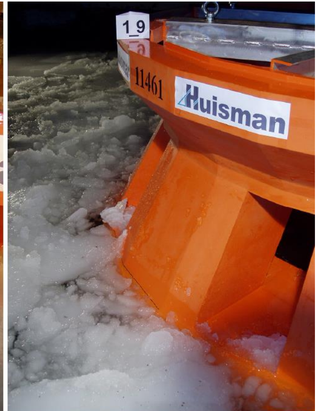
Model tests of JBF Arctic in ice (ice draft and transit draft)
