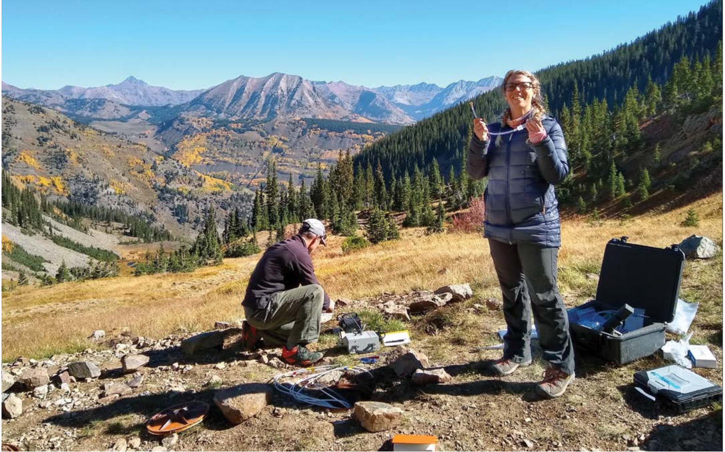
DANIELLA REMPE (RIGHT) INSTALLING EQUIPMENT FOR MONITORING GAS IN BEDROCK FRACTURES WITH ANDY MANNING OF THE U.S. GEOLOGICAL SURVEY IN RED WELL BASIN, NEAR CRESTED BUTTE COLORADO.
