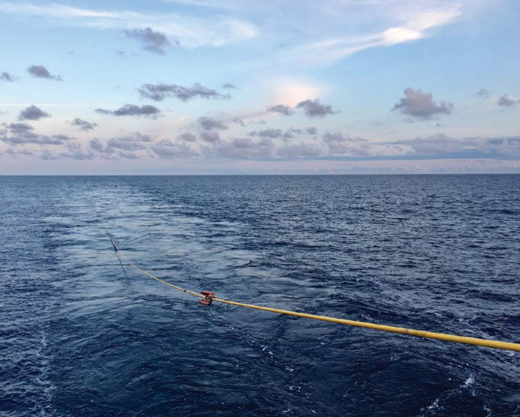
A SEISMIC STREAMER, WHICH IS USED TO IMAGE THE EARTH LIKE AN ULTRASOUND SCANNER, DURING SURVEYS ABOARD THE R/V MARCUS LANGSETH.
