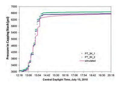
Wellhead pressure measured during and immediately after closure of the capping stack on the Macondo Well on July 15, 2010 as measured by pressure gauges installed on the capping stack (PT\_3K\_1 and PT\_3K\_2). The pink line denotes pressure simulated by the initial (square) reservoir model assuming a well with no leaks. Figure modified from Hsieh, P.A. (2011).
