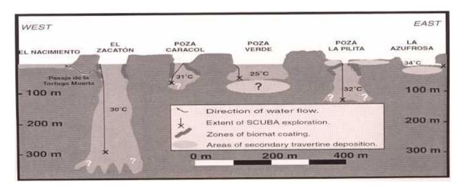
Figure 1: Generalized cross section of the cenotes of Rancho La Azufrosa. The limits of current exploration, locations of travertine deposition, and biomat-covered areas are represented.
