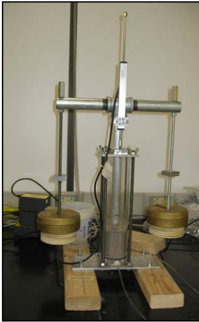
Figure A4.4: Resedimentation setup at unload.
