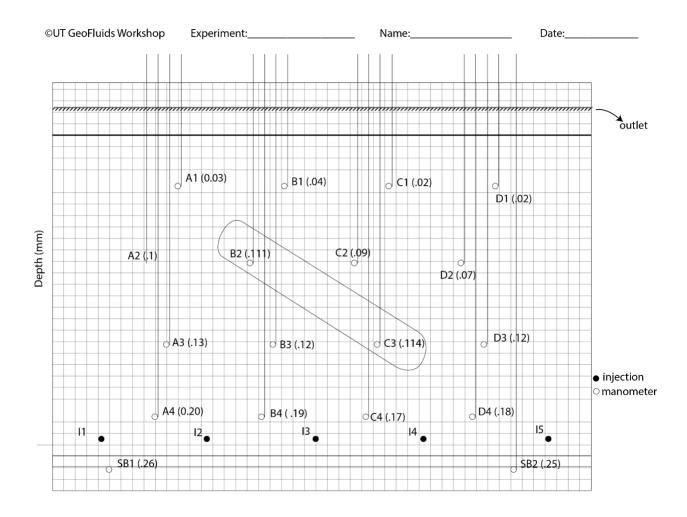
Figure 1: a) A tilting sandstone reservoir is surrounded by low permeable mudstone. Overpressure (ue, PSI) is shown in parentheses.
