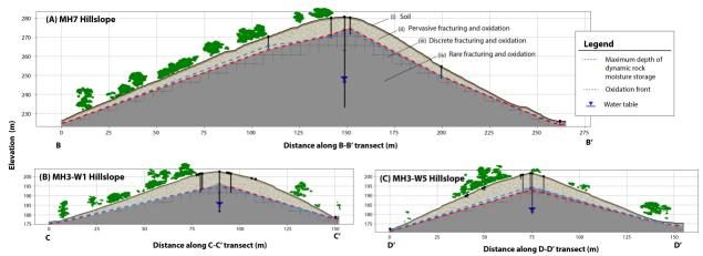
This figure is a summary of patterns of weathering and water storage across study hillslopes, namely MH7 (A), MH3-W1 (B) and MH3-W5 (C). The dashed lines are interpolated depths between direct observations made at boreholes. Four layers are identified based on the extent of fracturing and oxidation.
