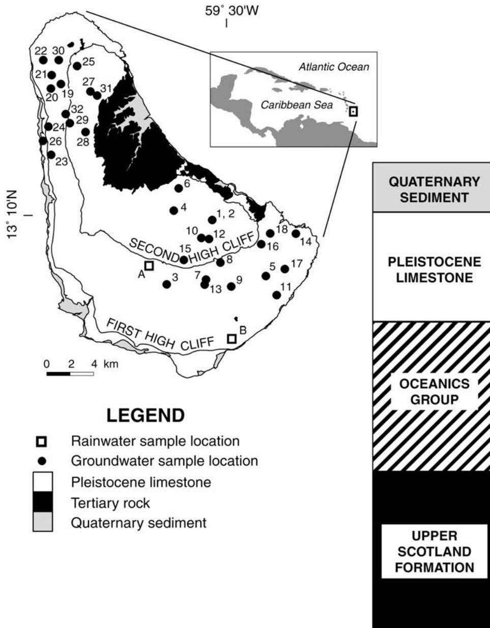
**Figure 3.** Geologic map of Barbados. The Pleistocene limestone that composes the aquifer occurs in the northern, western, and southern portions of the island. The Second High Cliff is approximately 30 m high and has been identified as a major site for discrete recharge to the underlying aquifer. The Tertiary rock outcrop is composed of the Oceanics Group and upper Scotland Formation. Adapted from Directorate of Overseas Surveys 1:50,000 geologic map (1983).
