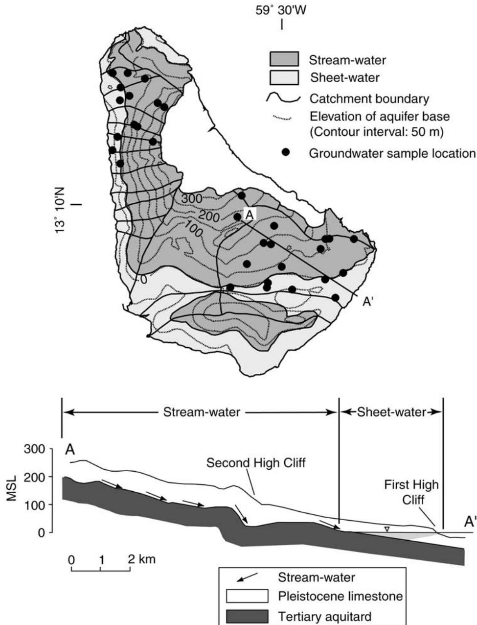
**Figure 4.** Hydrogeologic map of Barbados. The Pleistocene limestone aquifer is divided into several groundwater catchments due to the topography of the Pleistocene-Tertiary contact. The contours shown indicate the elevation of the base of the Pleistocene limestone. Adapted from *Stanley Associates Engineering Ltd.* [1978b] and *Barbados Ministry of Health et al.* [1991].
