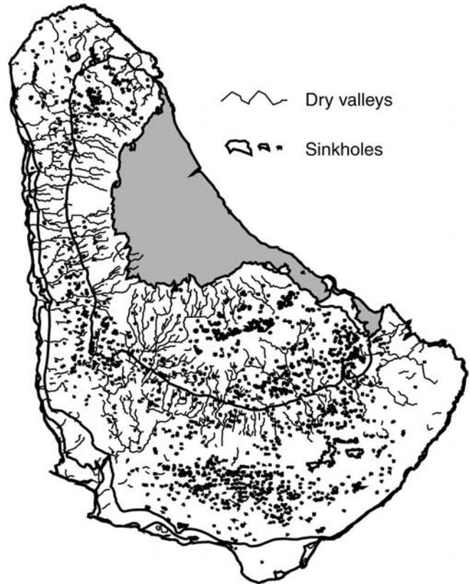
**Figure 7.** The major karst features on Barbados take the form of dry valleys on moderate to steep slopes and sinkhole depressions in flat areas, especially adjacent to the Second High Cliff. Adapted from Directorate of Overseas Surveys 1:10,000 topographic map series. Shaded area represents outcrop of Tertiary rocks.
