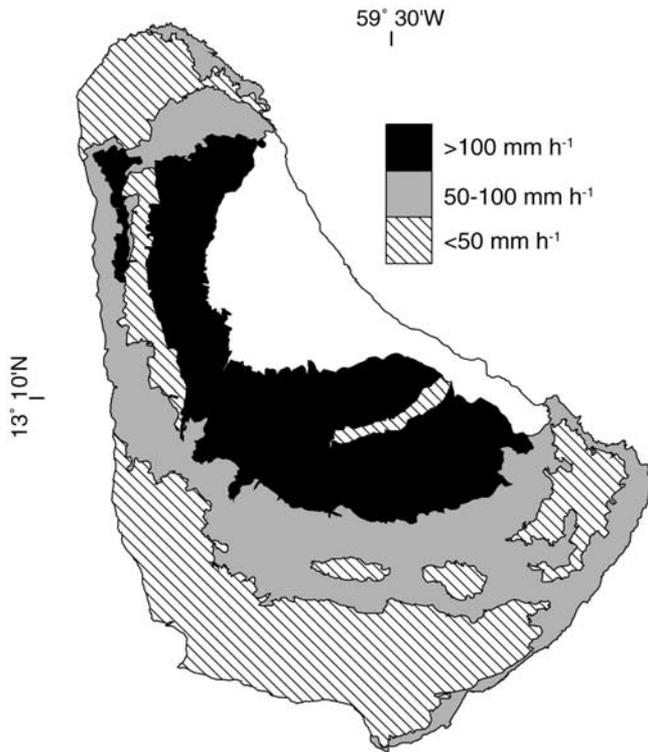
**Figure 6.** The infiltration rates of soils developed over the Pleistocene limestone aquifer. Barbados soil infiltration rates tend to increase with elevation. The most permeable soils occur above the Second High Cliff. Adapted from *Vernon and Carroll [1965]* and *Tullstrom [1964]*.
