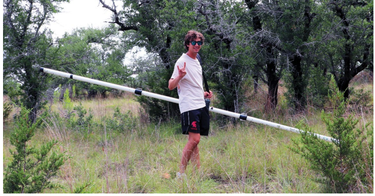
Above: Hawkins Borer conducting electromagnetic geophysical surveys at the White Family Outdoor Learning Center. Middle: Doctoral student Josiah Sananda demonstrating the vadose zone monitoring system. Below: Madison Fail (left) and Brooklyn Douglass (right) taking infiltration measurements at the WFOLC.
