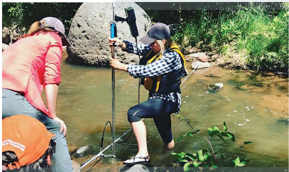
CLOCKWISE: RILEY WINEBARGER USES AN ACOUSTIC DOPPLER VELOCIMETER TO MEASURE THE FLOW OF THE JEMEZ RIVER WHILE KIMMY MCCORMACK LOOKS ON; ANNA TURETSKAIA AND LOGAN SCHMIDT ANALYZING THE GRAIN SIZES OF A SOIL CORE IN THE VALLES CALDERA; LISA THOMPSON, COLT KERNAN, RILEY WINEBARGER AND CHANCE BOLDUC LOOK AT CORE SAMPLES FROM THE EDWARDS AQUIFER ON THE WHITE FAMILY OUTDOOR LEARNING CENTER
