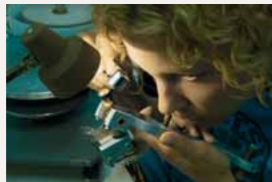
Undergraduate student Cristen Guest examines the polish on facets of a partially completed quartz gemstone. Photo by J. Jaworski, 2005.
