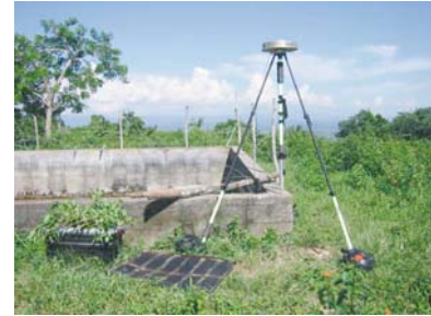
P. Mann (UTIG) and L. Pena (CODIA) reoccupied this GPS site on hilltop near La Vega, Dominican Republic, in October following the September 22 earthquake. This site has been occupied twice before over a period of 4 years.
