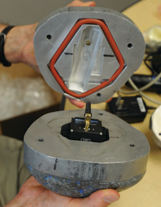
Johnson embeds accelerometers inside real rocks to make “smart rocks” that record the motions and forces a typical rock experiences under various stream flow conditions.
