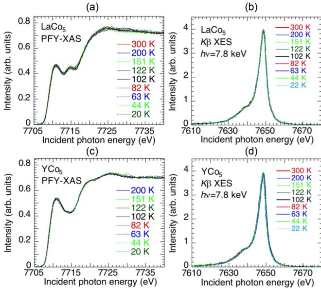
FIG. 4. Temperature dependence of (a) PFY-XAS spectra and (b)  $K\beta$  x-ray emission spectra for  $\text{LaCo}_5$  and (c) PFY-XAS spectra and (d)  $K\beta$  x-ray emission spectra for  $\text{YCo}_5$ .
