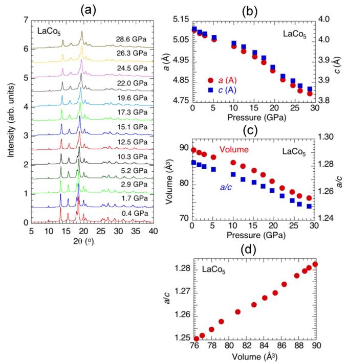
FIG. 1. Pressure dependence of (a) x-ray diffraction patterns, (b) lattice constants, and (c) volume and ratio of  $a/c$  for  $\text{LaCo}_5$ . In (d) dependence of the  $a/c$  ratio on the volume is shown.
