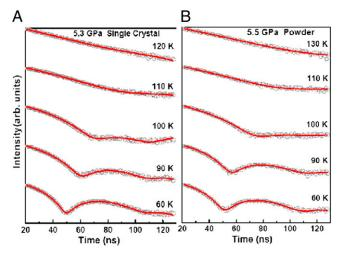
Fig. 1. Representative temperature-dependent SMS spectra of BaFe<sub>2</sub>As<sub>2</sub> in Ne pressure medium. (A) Single crystal at 5.3 GPa. (B) Powder sample at 5.5 GPa. O, experimental data; red solid lines, modeled spectra using the CONUSS program. Quantum beats in the spectra represent the occurrence of the magnetic fields and hence the AFM state, whereas the absence of beats (flat spectral feature) indicates the PM state.
