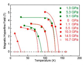
Fig. 2. Derived hyperfine magnetic fields of BaFe2As2 as a function of temperature at high pressures. Red symbols, powder in Ne medium; olive symbols, single crystal in Ne medium; solid symbols, AFM state; open symbols, PM state; solid lines, simple fitting to the data.
