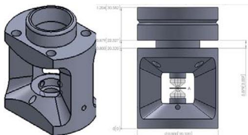
Figure 2. High-pressure and low-temperature cryostat system with miniature diamond anvil cell and Be windows for NRIXS.
