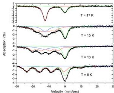
Fig. 1. Mössbauer spectra of EuS nanoparticles. Note the  $\text{Eu}^{3+}$  at  $\sim 0$  mm/s
