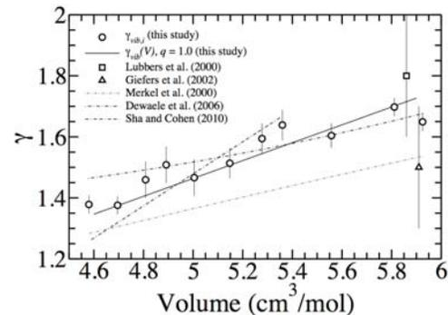
Figure 2. Volume dependence of the vibrational and total Grüneisen parameters for hcp-Fe from theoretical calculations and experiments [3].
