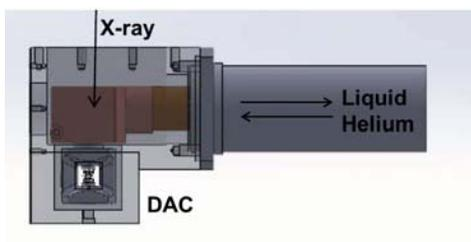
Figure 3. High-pressure and low-temperature cryostat system with two APD detectors collecting data.
