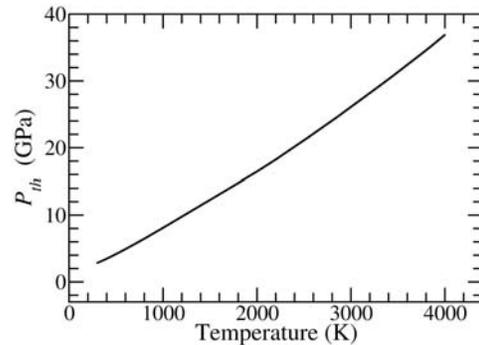
Figure 1. Total thermal pressure ( $P_{th}$ ) for hcp-Fe at a pressure of  $151 \pm 5$  GPa, accounting for electronic and anharmonic effects [2; 5].
