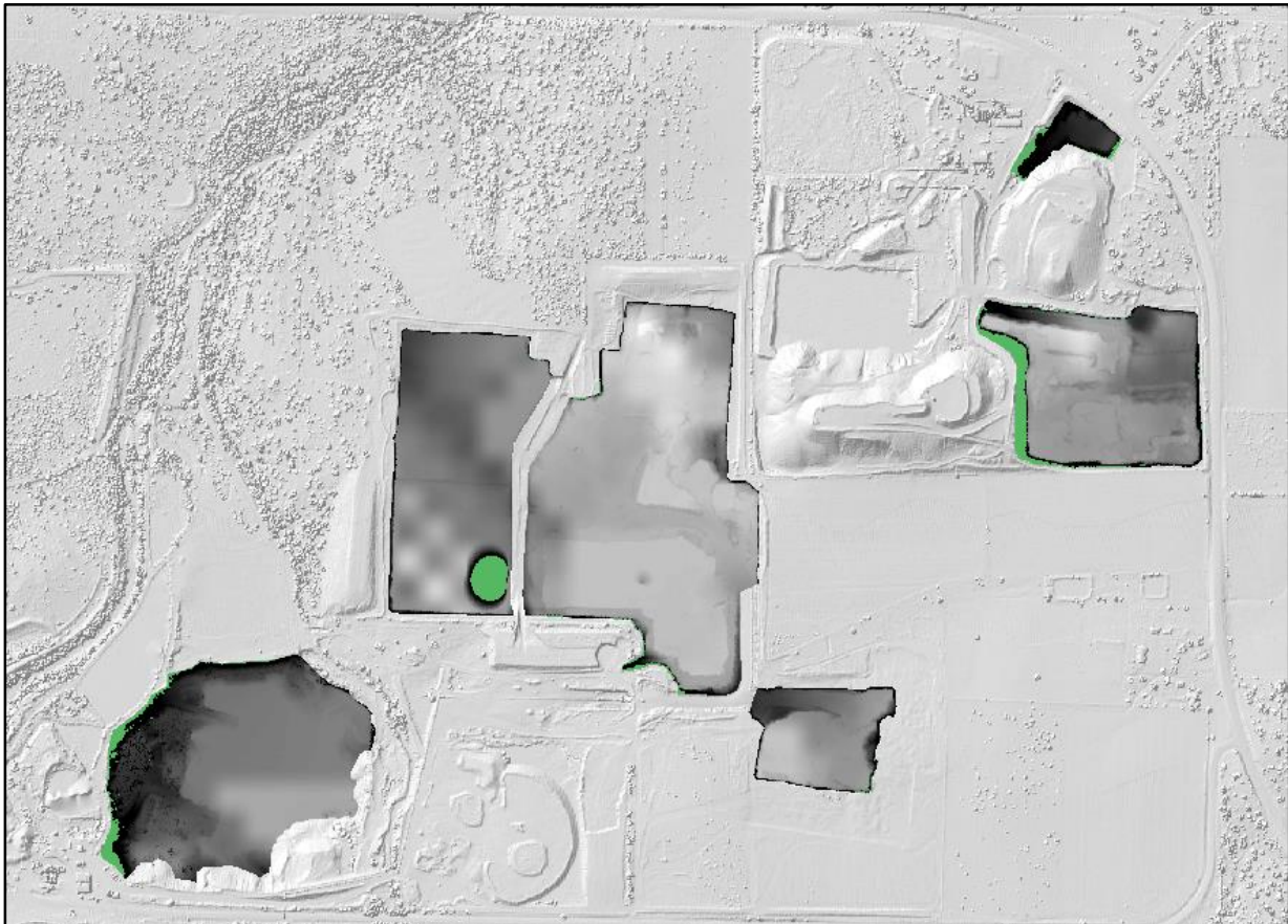
Figure 8. Raster showing areas that have a lower elevation post mining. Areas in green contained negative values that resulted from errors in the LiDAR data and from an incorrect definition of the edges of the pits and were set to null by the method described above.
