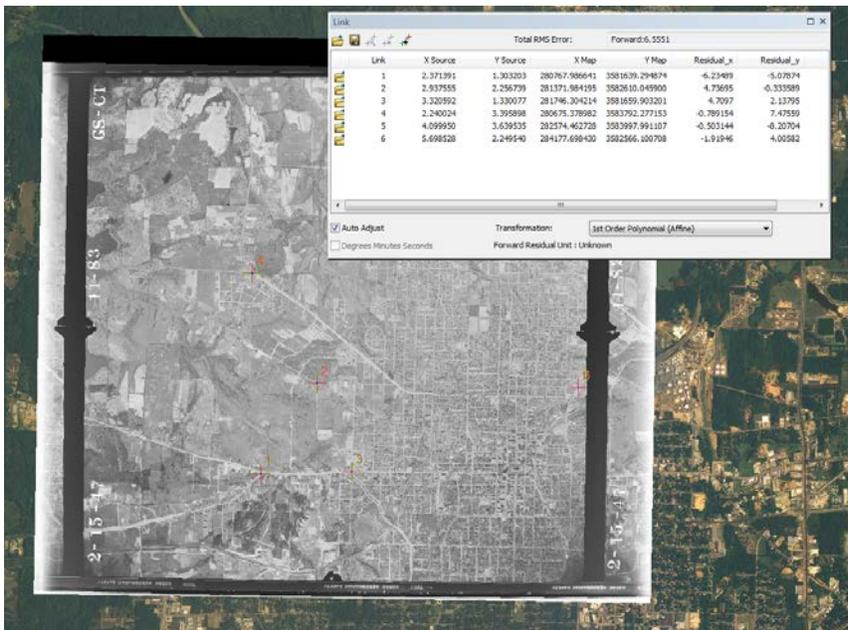
Figure 5. This is the 1947 aerial photo of the northeast corner of Tyler with its georeferenced links to the 2005 NAIP data.
