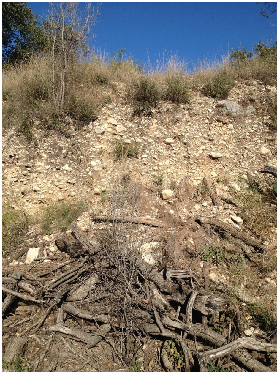
Figure 2. An example of the composition of the terrace labeled T2 (picture taken in field). It contains a fine matrix but still has the capacity for fluid flow.
