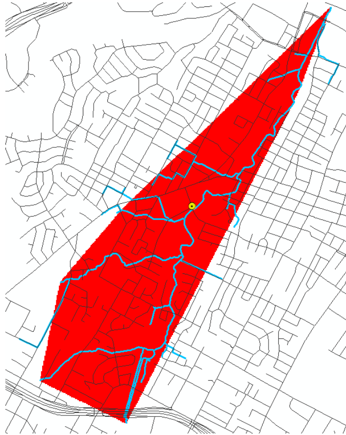
Figure 25: West Bouldin watershed after the Cut Fill tool was used to represent are that was flooded during the October flooding event taking not taking into account the storm drains.
