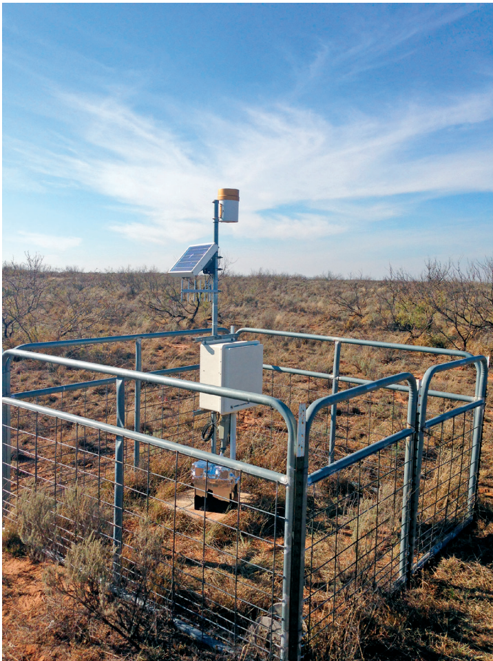
Typical layout of a TxSON soil moisture monitoring station (left). The soil pit (top right) is excavated and soil moisture sensors are inserted into the trench face (bottom right). The wires are routed below ground to a tripod containing additional meteorological sensors, a solar panel, and a data logger.
