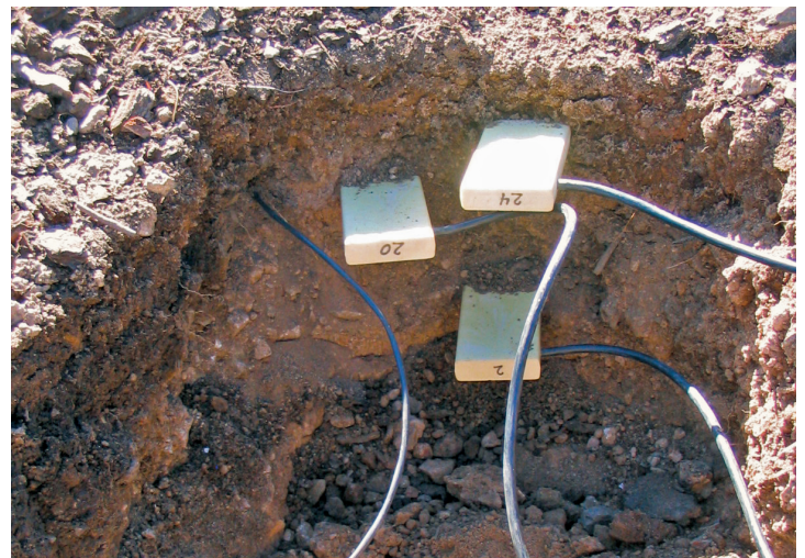
Typical layout of a TxSON soil moisture monitoring station (left). The soil pit (top right) is excavated and soil moisture sensors are inserted into the trench face (bottom right). The wires are routed below ground to a tripod containing additional meteorological sensors, a solar panel, and a data logger.
